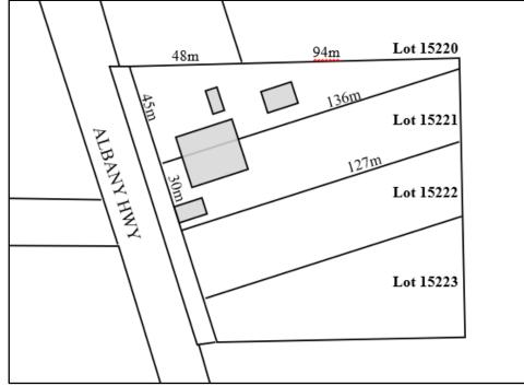
The development will consist of two dongas with one being 3.0m by 9.9m and the second one being 3.3m by 14.4m. They will be located behind the existing building.
