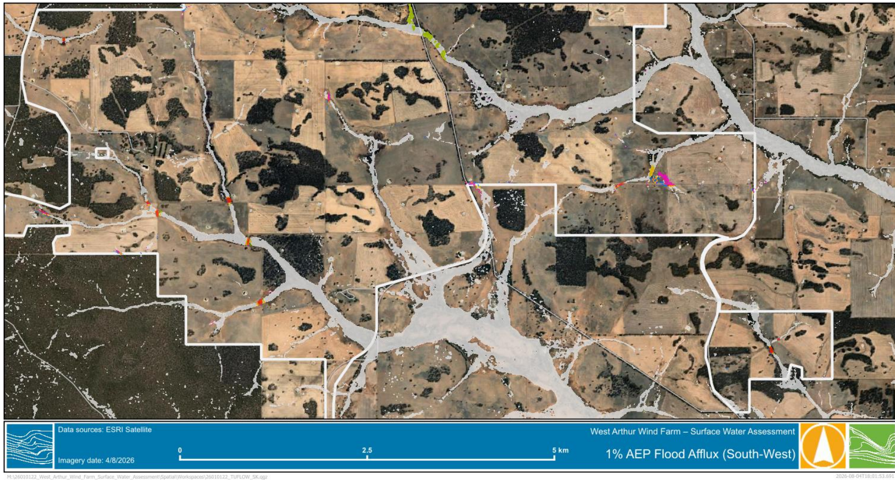
Figure 4-8 1% AEP Flood Afflux (South-West)
