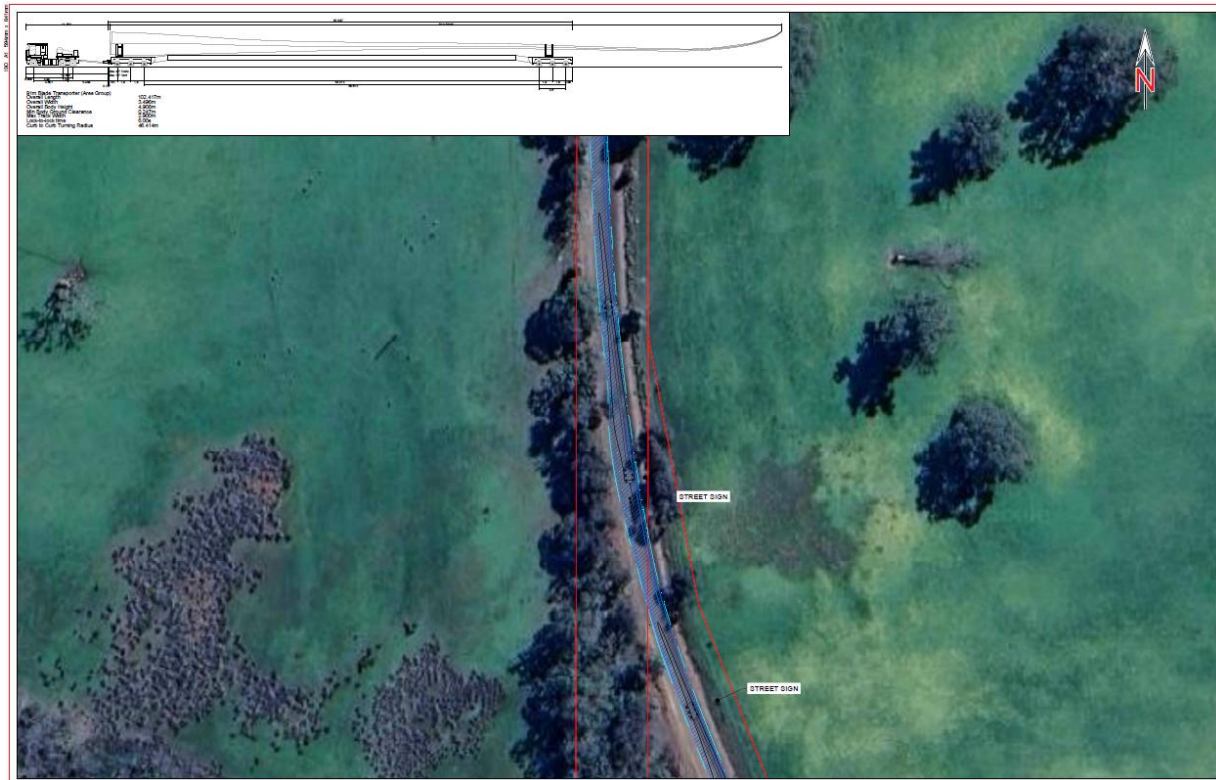
Figure 37 91m WTG blade swept path - Cordering Road North to north of Gibbs Road (source: Access Traffic)
