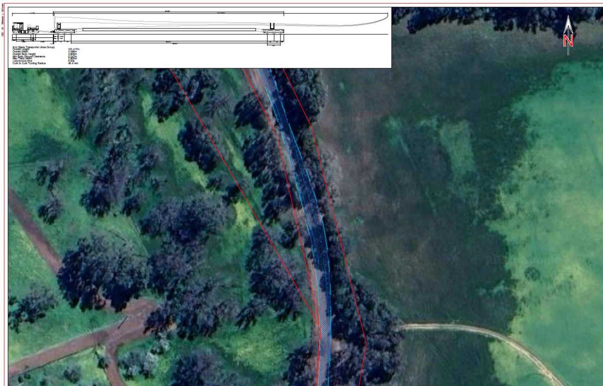
Figure 38 91m WTG blade swept path - Cordering Road North to south of Gibbs Road (source: Access Traffic)
